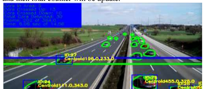
Fig.7. When the vehicle centroid crosses the imaginary line in ROI, the respective counter variables increase.
